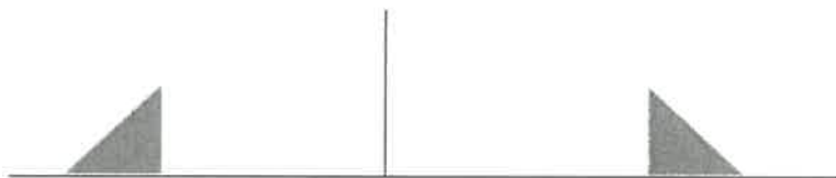
Figure .2 : Spectrum of the SSBSC wave
